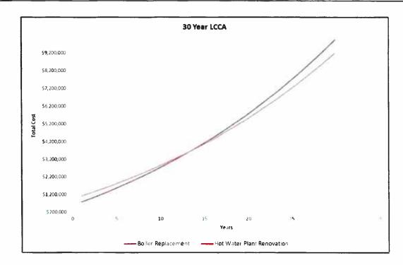
This calculation shows that after year 15 the total costs (annual energy and first costs) of replacing the boilers in kind would surpass that of the hot water plant renovation, with a 30-year total difference in energy cost of \$924,343! One other note to explain is the emissions onsite. Each year the hot water plant renovation project, at minimum, would produce 60 metric tons of carbon dioxide less than a boiler replacement in kind. Equivalent amounts would be:
